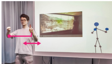
Figure 7: Example of an asymmetric bimanual gesture to control the playback position of a video.
