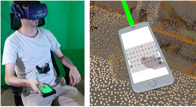
Figure 1: A mobile phone is used as VR controller with visual feedback of the user's thumb shown in VR
