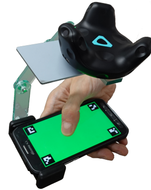
Figure 2: Mount holding mirror and VR tracker above the screen. The phone shows a green background with ArUco markers to optically locate the four corners of the screen.
