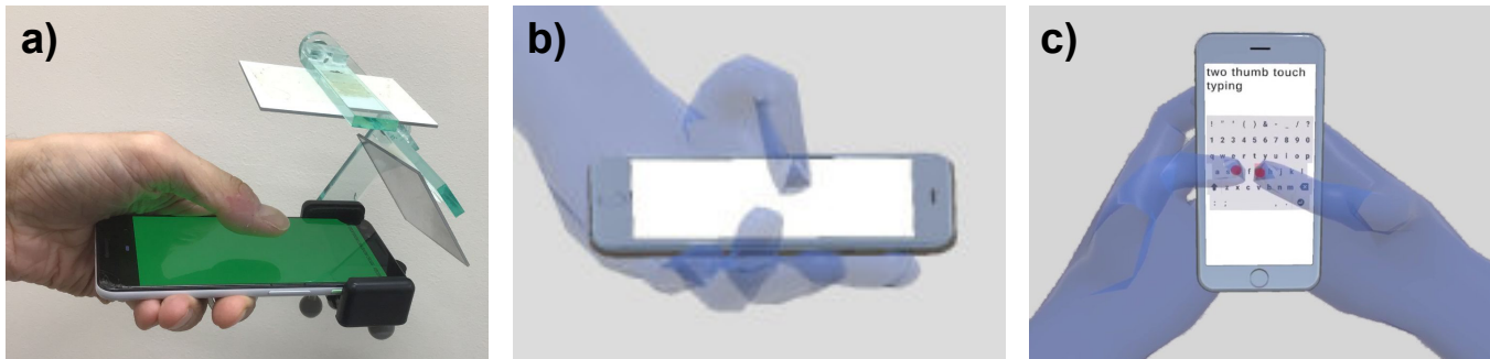
Figure 1: Phone-based fingertip-tracking system and hand models in VR: a) a custom mount with two mirrors captures the hand operating a phone from two different angles, 3D fingertip positions estimated with deep learning are used to control virtual hand models in VR (b) and c)).
