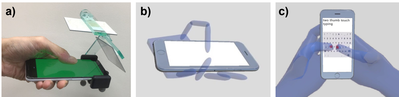
Figure 1: Phone-based fingertip-tracking system and hand representations: (a) a custom mount with two mirrors captures the hand operating a phone from two different angles, 3D fingertip positions estimated with deep learning are used to control different hand representations, e.g. (b) an abstract hand with stick-like fingers, (c) 3D hands with markers on fingertips to facilitate precise touch input such as typing on a phone keyboard.
