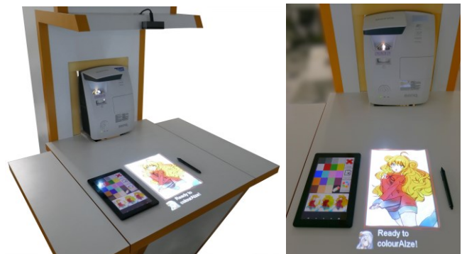
Figure 1. The ColourAIze system with an example of a semi-automatically coloured line drawing
