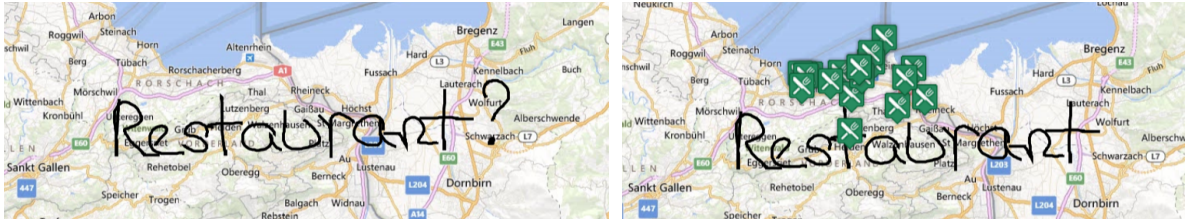
Figure 1: The QUERY? technique with implicit scope. When the question mark is appended to the query text, the results appear in the largest city close to the user ink.
