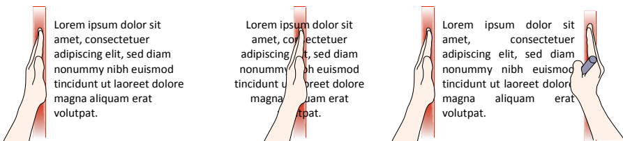
Figure 6.7. Chopping gestures for text alignment. Illustrated are left, centred and justified alignments.
