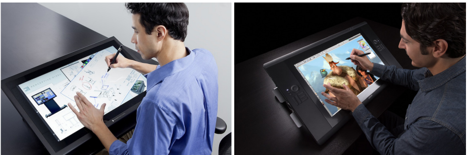
Figure 1.2: Two commercial surface systems with support for simultaneous pen and touch: Perceptive Pixel’s Active Stylus screen (left) and Wacom’s Cintiq 24HD Touch (right)
