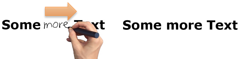
Figure 6.6. Insertion of handwritten text within text element. Text after the insertion point is gradually shifted to create space for writing.
