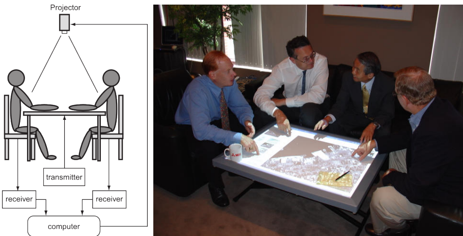
Figure 2.4: Schema of the DiamondTouch's signal loop (left) and a meeting scenario where the table is used (right)
