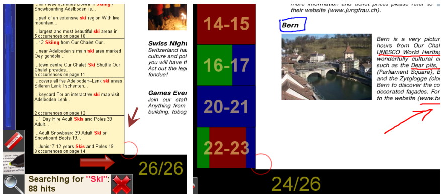
Figure 5.3: Text search tools. Dynamic page markers for search results with context snippets appearing on the side of the page (left) and bookmarks for annotated pages with stripes reflecting relative amount of strokes for each colour pen (right)
