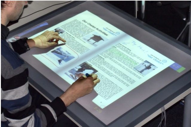
Figure 1: The active reading application running on a DiamondTouch tabletop [4] augmented with Anoto technology 4
